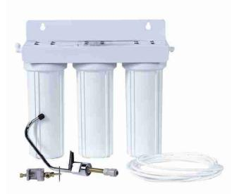
The UCTSTD-PR comes complete with NSF approved quick connect fittings, self piercing feed valve, NSF approved tubing, and long reach chrome faucet. The UCTSTD-PR also comes standard with a SF5-10 sediment filter, GAC10N grainular carbon, and PCTO/2 carbon block. Custom filter configurations are available upon request.
